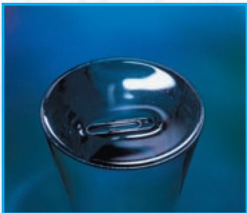
Paper clip floats on water because of surface tension.
